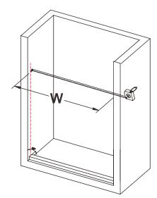
2. Your Upper Guide Rail [5] and Bottom Guide Rail [9] have been precut for your Shower model opening width, eg.60" for shower width. If W-width of your wall-to-wall opening is equal to the size of your Shower model, it is unnecessary to cut the Upper Guide Rail and Bottom Guide Rail and you can continue to Next Step3.
