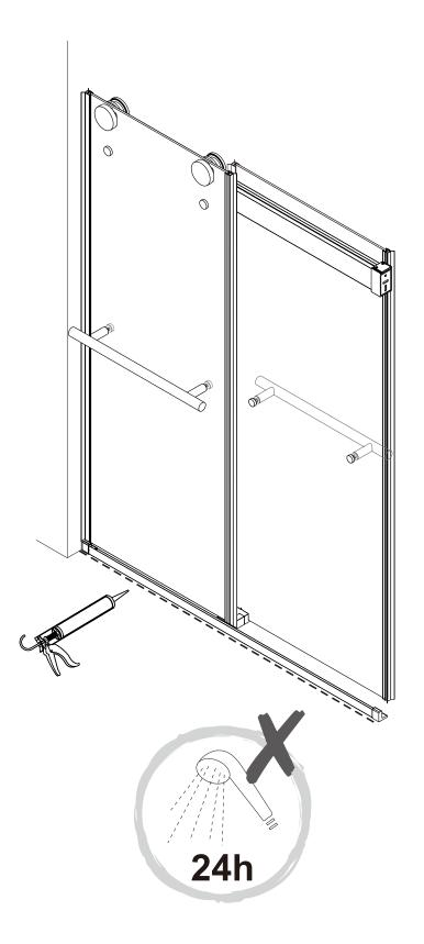
Do not use the shower enclosure for at least 24 hours in order to allow the silicone sealant to cure fully.
