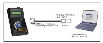
Application 2 Send Trilogy Lock Programs from PC to AL-DTM for transfer to multiple Digital Locks OR use the AL-DTM to retrieve system activity reports from locks to be transferred to the PC.
