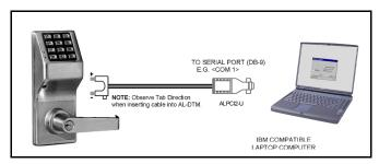
Program the Lock directly using a PC or Application 1 Laptop
