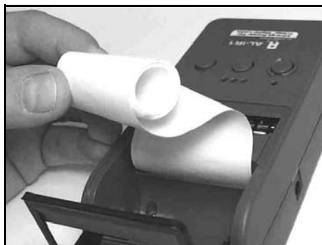
While pushing paper into slot, hold down the ▲ button until paper emerges. If paper jams, pull backwards VERY slowly.
