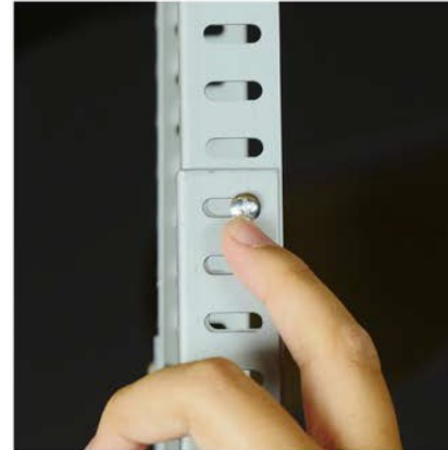
11. As needed, use an additional screwdriver to fasten the L-bracket.
