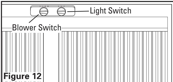
**NOTE:** On installation where a One (1) speed blower is utilized, all blower control speeds operate at the same speed. On installation where a Two (2) speed blower is utilized, the Medium and High speeds operate at the same speed.
