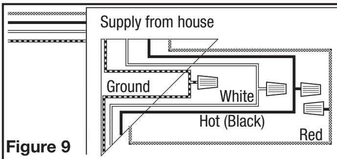
**NOTE:** The fan's receptacle wires might need to be pulled outside compartment for connection. Only pull the three loose wires outside of compartment. Additional wires will be present.
