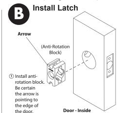
② Install latch and rotate the latch tongue \*\* to change handing. (See page 1 for handing)
