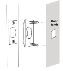
Attach the strike plate to the door jamb using 3/4" long wood screws.
