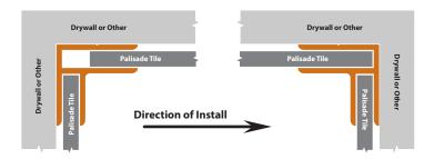
Next, determine the length of the tile section. Measure from the inside lip of the previously installed tile to the inside edge of the pre-installed trim. See image at right for details. In this case, the length to cut the final tile in the row is 4-3/4-inches (image 19).
