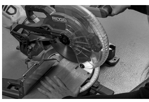
Cut away the notch with a miter saw.
