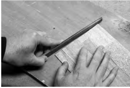
Proper position for squaring up an edge or smoothing a rough spot
