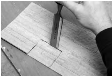
Cutting the inside edge with chisel
