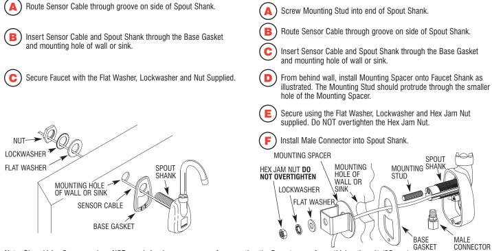
Note: Sloan Valve Company does NOT supply hardware necessary for mounting the Faucet on surfaces thicker than 1" (25 mm).
