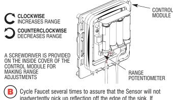
inadvertently pick up reflection off the edge of the sink. If reflection occurs, adjust Range Potentiometer counterclockwise very slightly and again cycle Faucet. Repeat adjustment procedure until desired range is achieved.
