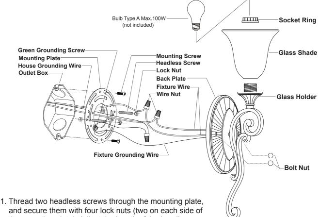
and secure them with four lock nuts (two on each side of the mounting plate). Adjust the length of the headless screws if necessary.
