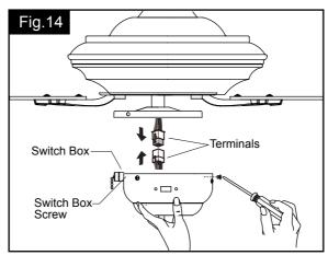
Connect the two terminals respectively from the motor and switch box.
