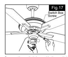
Secure the switch box with the switch box screws.
