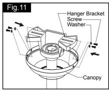
Attach the canopy to the hanger bracket, then secure it with four screws and washers.
