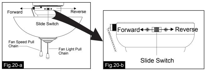
The slide switch sets the direction of fan rotation. Select the direction of fan rotation you need by sliding the switch. Push the slide switch left for "Forward" and right for "Reverse".
