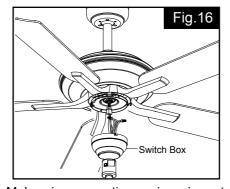
Make wire connections using wire nuts:
