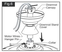
Insert the Downrod into the Collar. Slide Hanger Pin through holes of Collar and Downrod.
