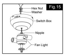
Thread the wires through the center hole of switch box. Attach the switch box onto the fan light with the nipple through the center hole of switch box, then secure it with a washer and hex nut.
