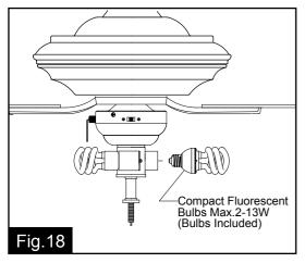
Install bulbs (included). See relamping label at socket area or packaging for maximum allowed wattage.
