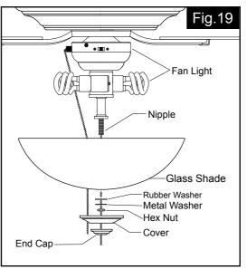
Install the glass shade, rubber washer and metal washer upward through the nipple and secure with hex nut. Then attach the cover to the glass shade and secure it with end cap.
