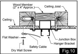
Attach the loop at the end of the safety cable to the ceiling surface, then secure it with a flat washer and dry wall screw. Make sure the flat washer and dry wall screw are covered by the fan canopy.
