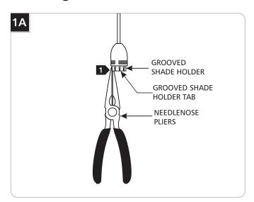
If the Martini glass fits tight onto the fixture, then carefully bend the grooved shade holder tabs in slightly with the needlenose pliers. If it fits loose, then carefully bend the grooved shade holder tabs out slightly with the needlenose pliers.
