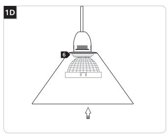
6 Hold the lamp against the glass with the thumb and push the lamp pins all the way into the socket holes; simultaneously push the Martini glass metal ring onto the grooved shade holder.
