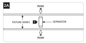
1 Place the separator (provided in the package) between the fixture wires. Push the wires toward each other until the fixture wires snap into the separator.
