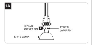
Push the lamp pins all the way into the socket. Improperly installed lamp may drop out.
