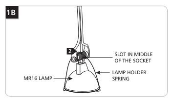
2 Hook one end of the lamp holder spring (provided with the package) onto front of the MR16 Lamp. Wrap the spring over the slot in the middle of the socket and hook the other end onto front of the MR16 lamp.
