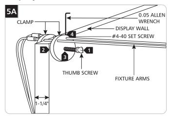
**NOTE**: The Lite Clamp can be clamped on maximum 1-1/4" thick display wall.
