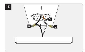
**5** Ground the mounting plate in accordance with local electrical codes.
