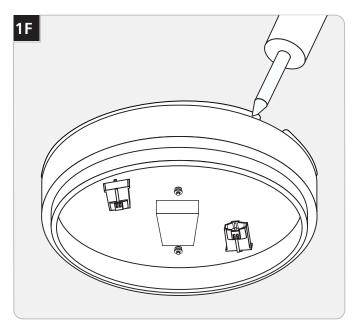
**10** For wet location installation, caulk around the mounting base with waterproof construction sealant.
