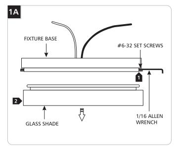
While supporting the glass shade, loosen (**Do Not Remove**) the four #6-32 set screws on mounting plate with the 1/16 Allen wrench.
