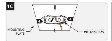
Secure the mounting plate to the electrical box with 2 #8-32 screws.
