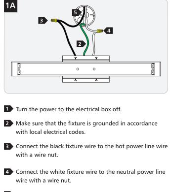
Secure the backplate to the electrical box with the two long #8-32 screws provided.
