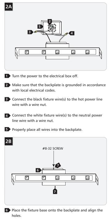
**7** Replace and tighten the #8-32 screws.
