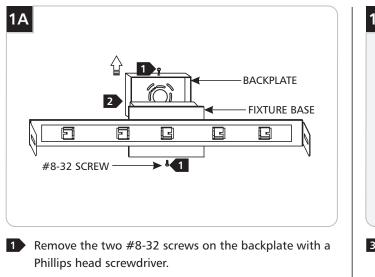
2 Remove the backplate from the fixture base.
