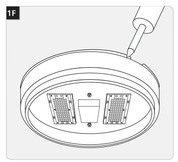
For wet location installation, caulk around the mounting base with waterproof construction sealant.
