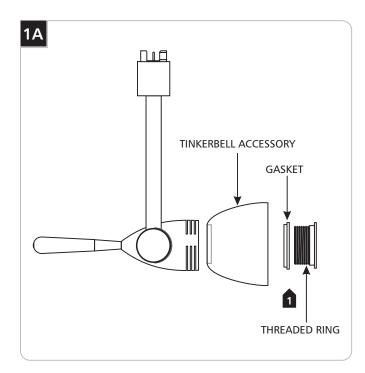
1 Place the threaded ring into the gasket and the Tinkerbell Accessory.
