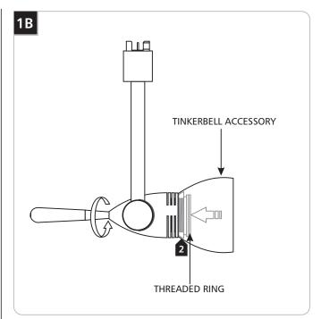
2 Screw the threaded ring completely to front of the fixture.
