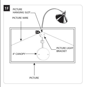
14 Hang the picture wire in the picture hanging slot on the picture light bracket.
