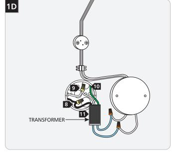
8 Connect the black transformer wire to the 120 volt power line wire with a wire nut.
