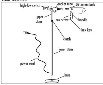
1. Screw lower stem of lamp on to base (Fig. A)
