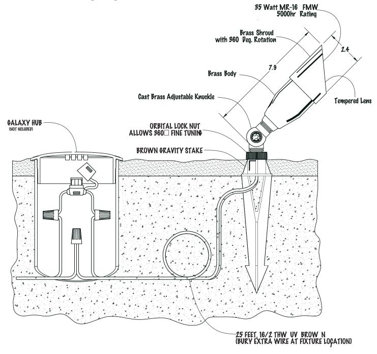
Glare / Light Trespass Shroud: Angled / Reduces incidental fixture glare Lenses Tempered Glass / High strength True Aim Knuckle: Brass two piece with thumb screw / Allows fo
