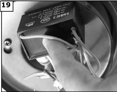
Remove the double sided sticky tape and stick the capacitor to the switch cap plate.
