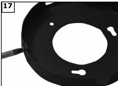
Remove the 3 screws from the switch cap plate and save for later use.
