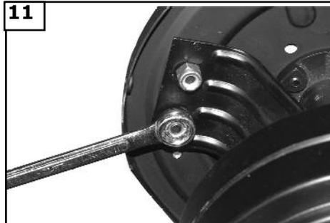
Lift the motor bracket so that the threaded studs on the mounting plate protrude through the slots in the motor bracket. Securely tighten the locknuts onto the threaded studs.
