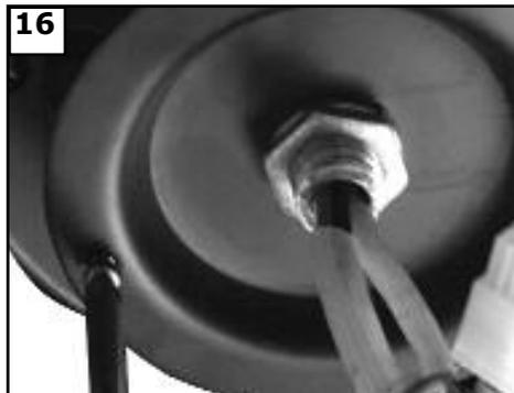
Loosen 2 screws and remove 1 screw from the motor plate and save.
