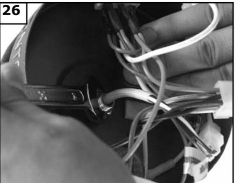
Remove the hex nut and lockwasher from the switch cap.
