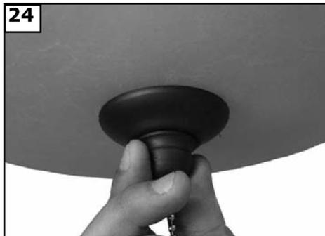
Place glass onto the fitter by threading the light kit pull chain through the glass, rubber washer, hex nut, finial cap, and finial. Tighten the finial securely by hand.
