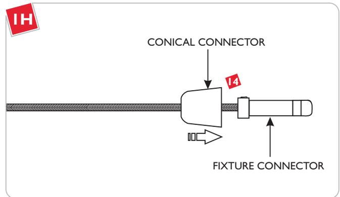
14 Slide the conical connector over the fixture connector. To install the fixture, refer to the instructions provided with the system.
