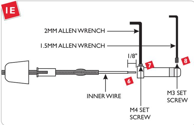
6 Strip 1/8" from end of the inner wire. **Make sure that the stripped portion is not greater than 3/16".**
