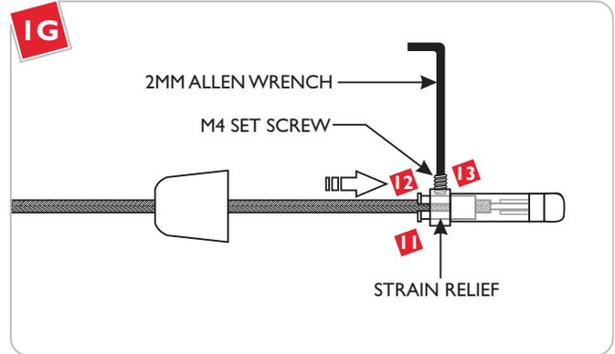
11 The strain relief slots should be rotated 90° away from the M4 set screw.
