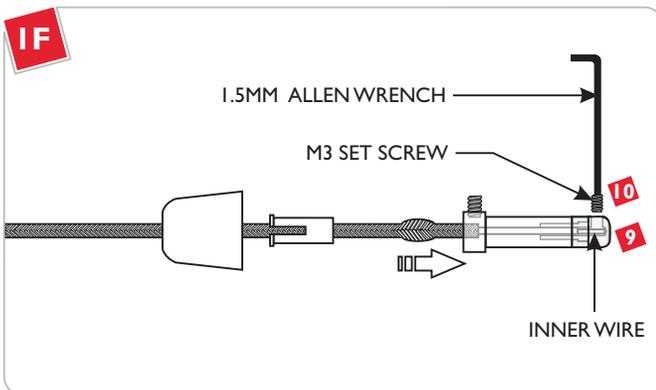
9 While inserting the inner wire into the connector look through the set screw hole to make sure that the stripped portion of the inner wire contacts end of the connector.
