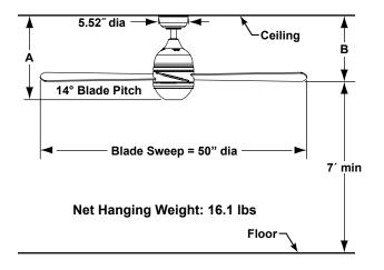
Fan must be attached to a securely anchored electrical junction box capable of withstanding a load of at least 50 lbs.
