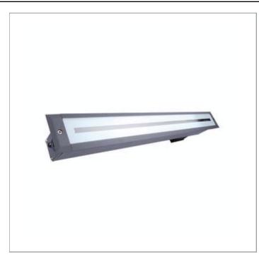
Linear T5 up-light. 120V input, integral ballast. Tempered safety glass lens. Symmetrical diffuser of anodized aluminum. Cast aluminum outer trim with powder coat finish. Cast aluminum metal body with powder coat finish. PVC mounting housing included.
