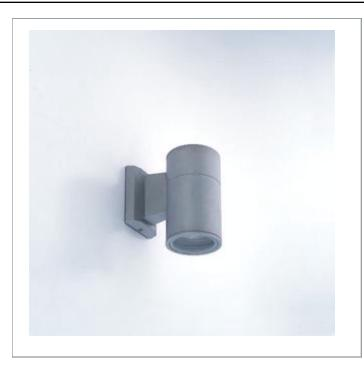
Cylinder wall light for down-lighting. Exterior grade. Cast aluminum construction with powder coat paint. Clear glass lens, unit is completely enclosed.
