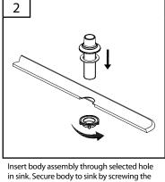
in sink. Secure body to sink by screwing the mounting nut from the underside of the sink clockwise. Hand tighten only.
