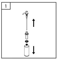
Remove the bottle. Separate soap dispenser head from flange body assembly.
