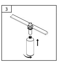
Screw bottle clockwise onto body assembly shank.
