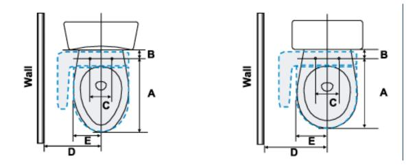
Note: Some styles of toilets may not allow the Washlet C110 to be installed due to certain contours near the tank and bowl area (see figures below). In the figure on the left side below, dimension D does not allow for enough open space to accommodate the minimum width of 11 inches.
