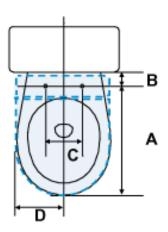
Note: Some styles of toilets may not allow the Washlet E200 to be installed due to certain contours near the tank and bowl area (see figures below). In the figure on the left side below, dimension D does not allow for enough open space to accommodate the minimum width of 9 inches.
