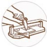
Measure tiles to be cut carefully and mark with a pencil or felt-tip pen. Make straight or diagonal cuts with a tile cutter, curved cuts with a nipper (chipping away small pieces for best results), full-length curved cuts with a rod saw. Sharp-cut edges may be smoothed with a carborundum stone.
