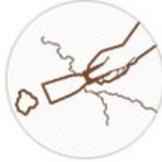
Tile may be installed over most structurally sound substrates, if they are clean, smooth, dry and free of wax, soap scum and grease. Any damaged, loose or uneven areas must be repaired, patched and leveled. Remove any moldings, trim, appliances, etc., which could interfere with installation. Door jambs may be undercut for tile to slip under.
