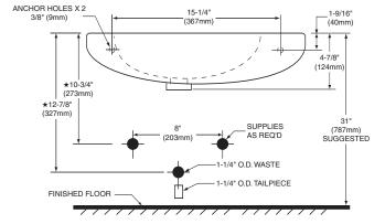
DIMENSIONS SHOWN FOR LOCATION OF SUPPLIES AND "P" TRAP ARE SUGGESTED. PROVIDE SUITABLE REINFORCEMENT FOR ALL WALL SUPPORTS. WALL ANCHORS AND MOUNTING FEATURES TO BE FURNISHED BY OTHERS. FITTINGS NOT INCLUDED AND MUST BE ORDERED SEPARATELY.
