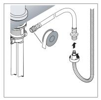
Place a hose washer in the elbow. Install the handshower (not included). Guide the handshower and elbow into the holder.
