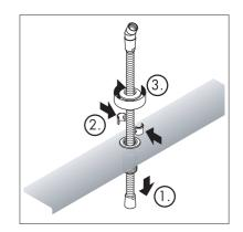
Seal the threads on the inlet end of the high pressure hose with Teflon tape. Install this end of the hose to the outlet on the mixing valve.
