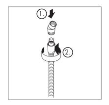
From the top, thread the hose through the handshower holder escutcheon and handshower holder (1). Snap the two halves of the hose insert around the hose (2). Press the hose insert down into the holder. Install the escutcheon (3).
