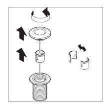
Place the handshower holder and sealing ring in place on the mounting surface (1).
