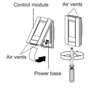
NOTE: Keep the thermostat's air vents clean and unobstructed at all times.
