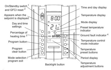
$<sup>^{1}</sup>$  Place the switch in Standby to cut power to the heater when not in use (e.g., in the summer). This will not affect the time and temperature settings.
