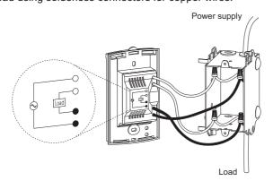
Insert the floor sensor cable through one of the two openings on the base and connect the sensor wires to terminals 1 and 2 (no polarity).
