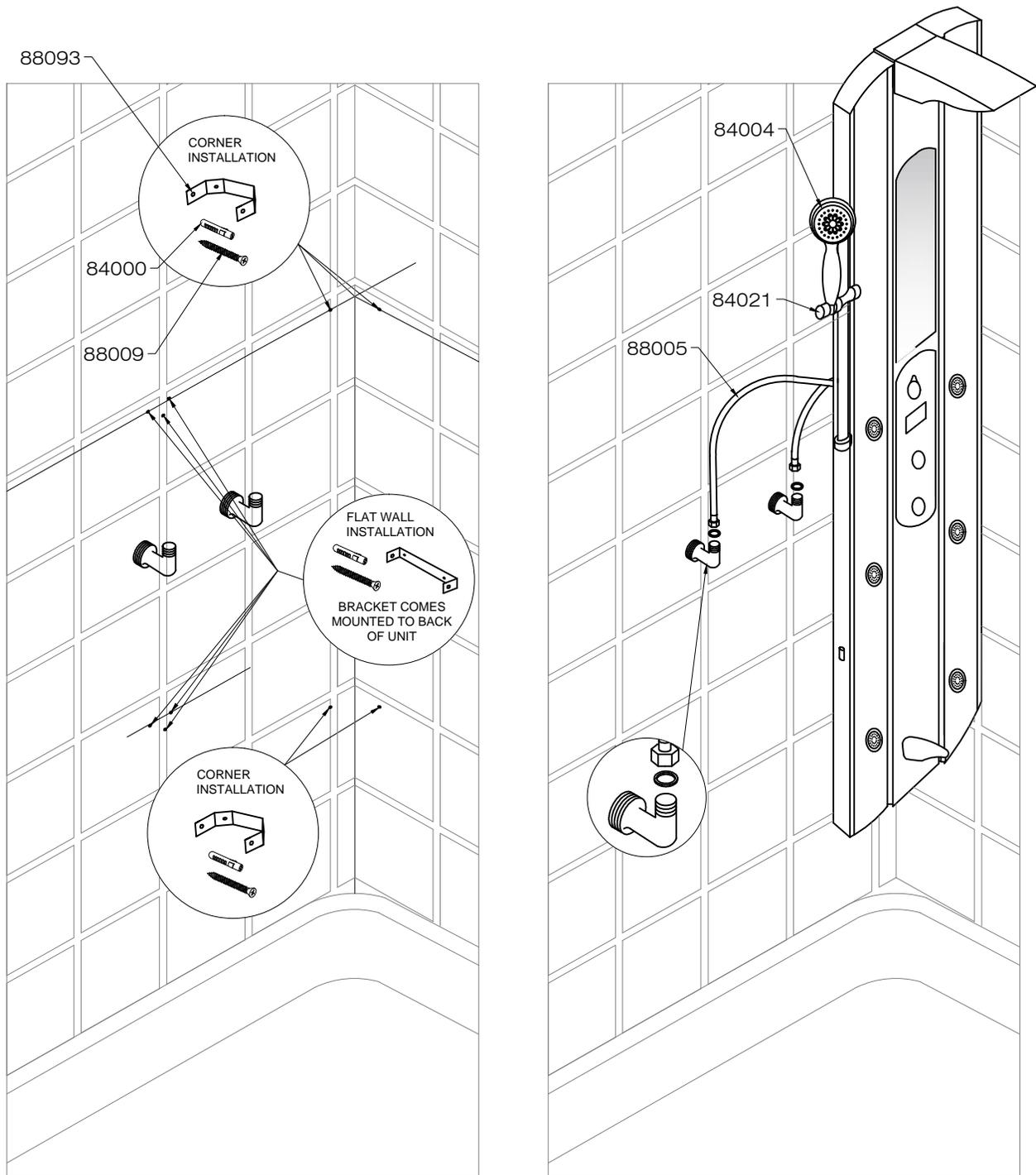
Save time and frustration: if turning the volume/temperature control handle gives both hot and cold water, but the water does not mix, the hoses may have been connected to the incorrect supplies. Please disconnect the hoses, reattach them to the correct supplies and test the unit.
