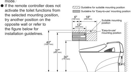
Attach the remote controller hanger to the wall.
