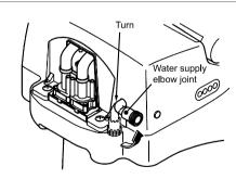
Turn the elbow joint so that it is facing downwards at a 90° angle.
