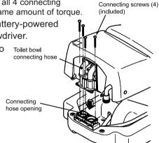
Tentative tightening of the screws. Align the main unit with the 4 screw holes on the toilet bowl fixture and tentatively fasten with the 4 bolts provided.
