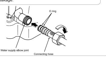
Connect the connecting hose to the water shutoff valve. \* Make sure that the hose is not bent or twisted before connecting it. Packing washe Water shutoff valve
