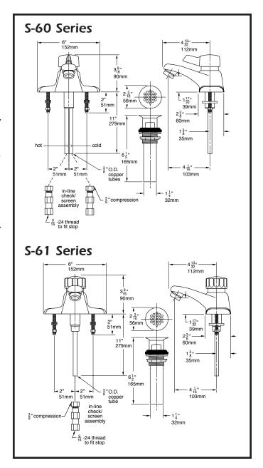
Remove handle (LL-104), loosen nut (LL-6) and turn stem (LL-1A) to desired maximum temperature (110°F recommended). Turn limit stop washer (LL-23N) clockwise until a positive stop is reached against back of faucet. Tighten nut (LL-6), replace and tighten handle (LL-104). Faucet will operate from the full cold position to the maximum hot temperature that has been set.
