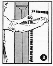
Note: The flat side panels are not interchangeable, but are clearly marked on the backs as to TOP and RIGHT or LEFT side. These panels are slightly taller than the corner panel forming an overlap and water tight seal.
