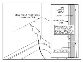
Use the 3/8" drill bit to enlarge the 3/16" pilot holes through the Swanstone wall panel or other wall material. Only drill the 3/8" holes through the thickness of the wall panel. Do not drill into the 2 x 6 inch wall support.
