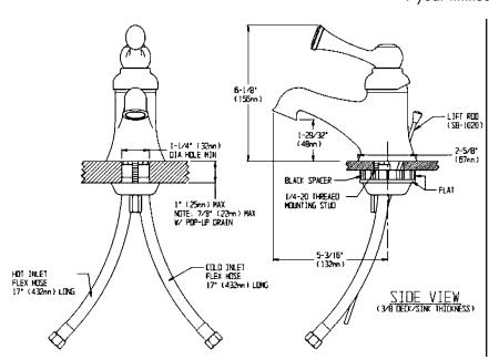
NOTE: 1. All dimensions are in inches (millimeters) unless otherwise specified and are subject to change without notice. 2. Flex hoses have 3/8 compression female threaded connections. 3. Use black spacer for deck/sink thickness of 3/8 and under (see side view above).
