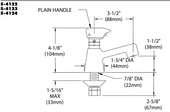
NOTE: All dimensions are in inches (millimeters) unless otherwise specified and are subject to change without notice. Inlet is sized for either cou-152 pling or sweat connections. Unless otherwise specified, inlet is 1/2" NPSM.
