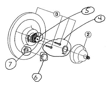
MOUNTING SCREWS+CAM+DIVERTER ASSEMBLY 2303-1210 MOUNTING SCREWS
