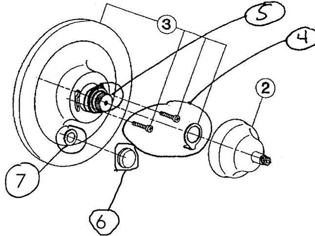
MOUNTING SCREWS+CAM+DIVERTER ASSEMBLY
