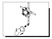
5. FOR TUB SPOUT INSTALLATION Install tub spout. Thread spout onto threaded connection clockwise until the spout becomes flush with the finished wall. Thread sealant may be required depending on your installation method. All thread sealants may be found at your local hardware store.
