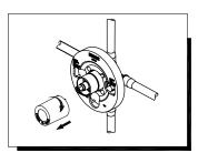
Before installing escutcheon, remove the plastic cap from plaster guard by twisting cap in a clockwise direction. Remove the screw from the
