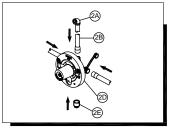
SHOWER ONLY SUPPLY CONNECTION LAYOUT Wrap plumber's tape around pipe threads in a clockwise direction.
