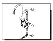
For Tub and Shower Combinations: Turn on Hot and Cold water supply lines allowing water to flow from tub spout outlet (4B) until all foreign matter has cleared the line. For Shower Only Combinations: Turn on Hot and Cold water supply lines allowing water to flow from shower outlet (4A) until all foreign matter has cleared the line.
