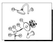
8. Install escutcheon (8A) onto valve and then insert screws (8B) to attach to valve body. Insert screw (8C) into inverter. Place handle seat (8D) onto the valve and secure with set screw (8E). Install handle assembly (8F). Attach shower (8G) to shower
