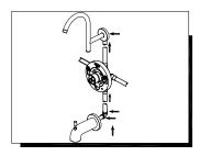
Place handle on valve stem and turn handle to full on mixed position. Turn on hot and cold water lines to full open for one minute each. Check for leakage. Shut off water at faucet. Remove the handle.
