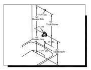
1. SHUT OFF WATER SUPPLY. Verify that the hole sizes and positions of holes in the wall are correct. Recommended component measurements A.Shower and / or spout outlet hole: 1-1/4" diameter.
