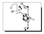
3. FOR SHOWER ARM INSTALLATION. Insert the long end of the shower arm (3B) through the flange (3A) then wrap plumber's tape to both sides of shower arm. Screw long end of the shower arm into pipe elbow inside the wall.
