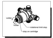
7. ADJUSTING WATER TEMPERATURE ADJUSTING WATER TEMPERATORE
