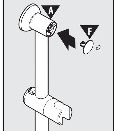
Attach Bracket Caps (F) to Brackets (A), one for each end.
