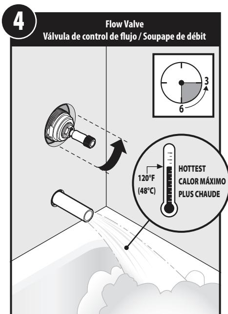
If temperature is over ( $>$ ) 120° F go to C1. If less ( $<$ ) 120°F, turn off flow valve (3 to 6 clockwise) and replace plaster caps.
