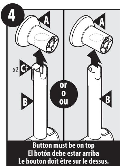
Install Slidebar (B) into each end of Brackets (A). Installation may include Slidebar Caps (C) for certain models. **Note:** the button on the adjustable slider must be facing up during bracket attachment.
