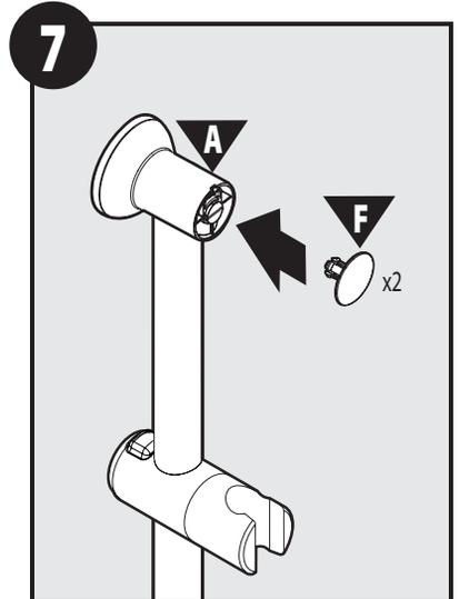
Attach Bracket Caps (F) to Brackets (A), one for each end.
