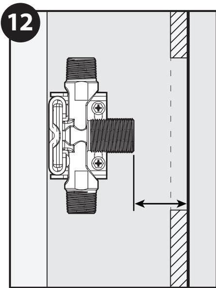
If distance is less than or equal to 2-1/8" (54mm), proceed to step 13. If distance is greater than 2-1/8", order 1" extension kit #155656.
