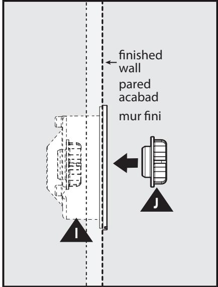
Tighten housing nut (J) until housing (I) is secure and does not spin on wall.
