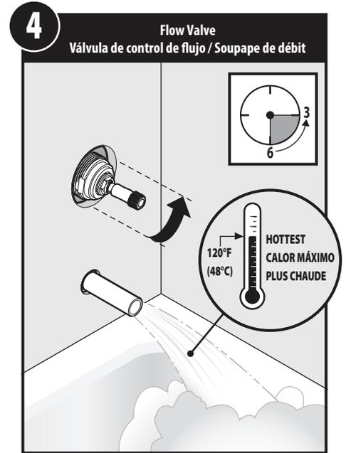
If temperature is over (>) 120° F **go to C1**. If less (<) 120° F, turn off flow valve (3 to 6 clockwise) and replace plaster caps.
