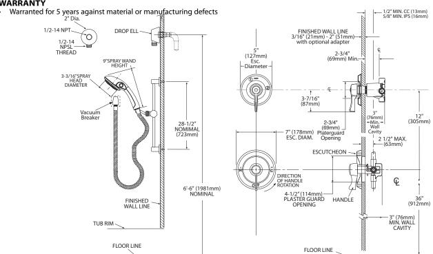
NOTE: This valve is not intended to be used as a shut-off valve. To prevent the potential of cross flow, check valves must be integral to the supply valve or installed in both hot and cold water supply lines. \*Refer to (ADAAG) guidelines or local codes for proper ADA installation.
