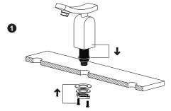
Fit O-ring 12 into the bottom groove of faucet body 11. Insert faucet body 11 into specified drill hole (1 ¼"- 1 ½") on the counter top. Install washer 13 and brass washer 14 to the threaded tail pipe of the faucet body 11 from underneath the counter top and then screw the fixing ring 15 to securely tighten the faucet body. Fix faucet body 11 correctly and install the three way connector 18 by screwing onto the threaded tail pipe of the faucet body 11.
