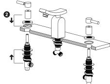
Install valve 9 into specified drill hole underneath the counter top. Place o-ring 4 into the base plate 3. Screw base plate 3 and the valve cover 2 into valve 9. Adjust the height and position of valve 9, then screw fixing ring 8 to tighten valve 9 underneath counter top securely. Install handle 1 to handle connector 5 of valve 9. Tighten set screw 21 with alley key and then place.
