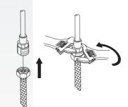
Apply pipe tape on threads of the inlet port. Tighten end of shank with wrench and slip hose into the inlet
